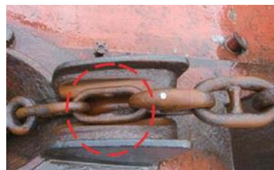
Worn link and missing of stud
