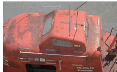
Poor condition of lifeboat hull
